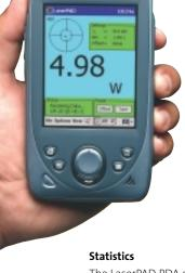
The LaserPAD PDA can perform complete statistical and power trend analysis for stability and drift measurements. From 40 to 2000 data points can be recorded and analyzed over a selected period of time for display on a strip chart or histogram plot.
